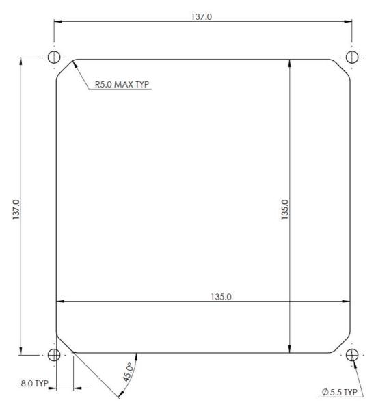
Figure 6: Recommended Panel Cut-out
