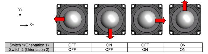
Figure 1 Mounting Orientations
