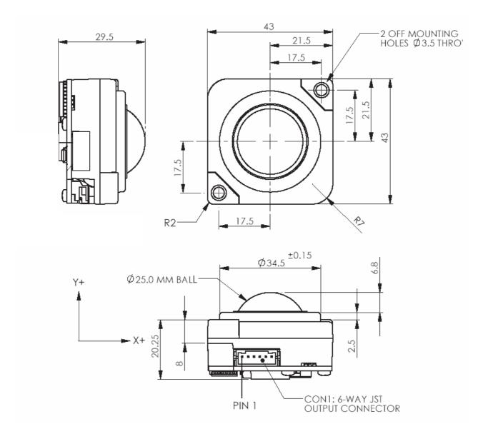
Dimensional drawing specifies factory default orientation. All dimensions are in mm unless otherwise stated.
