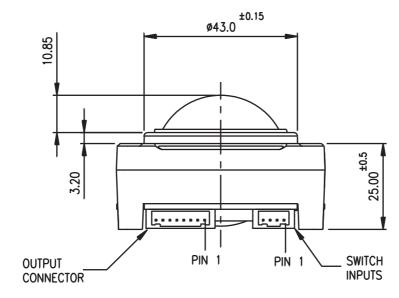
Dimensional drawing specifies factory default orientation. All dimensions are in mm unless otherwise stated.
