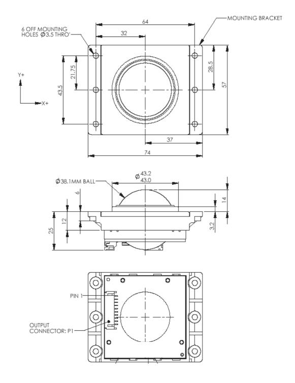
Dimensional drawing specifies factory default orientation. All dimensions are in mm unless otherwise stated.
