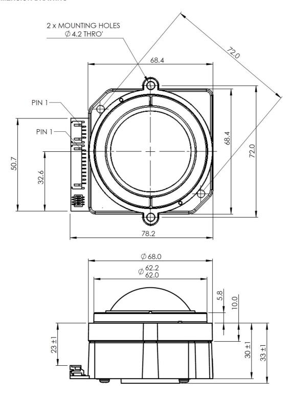
Dimensional drawing specifies factory default orientation. All dimensions are in mm unless otherwise stated.
